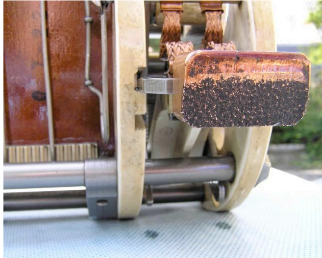
Figure 7 Aged Diverter Switch Contacts
