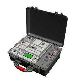
changer control unit enables remote control of the tap changer operation from the instrument's keyboard. The measurement is completed quickly on even the largest power transformers. Each vector group has a special measurement algorithm which is optimized for the fast stabilization of the test results.
