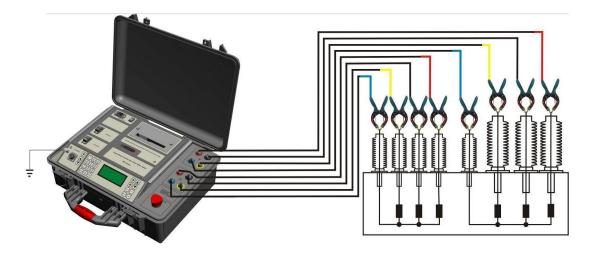
**Note:** It is important not to erroneously swap the HV and LV cables. If this happens, "Turns Ratio Too Low" warning message will be displayed, and the test will be interrupted in order to avoid dangerously high voltages.
